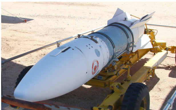
AIR-2A Genie nuclear air-to-air rocket on a MF-9 Transport Trailer; Source: Flickr.com/kitmasterbloke
